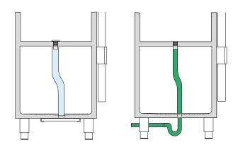
The drain diameter is  $1\frac{1}{2}$ ", therefore it is advisable to use a  $1\frac{1}{2}$ " drain pipe.
